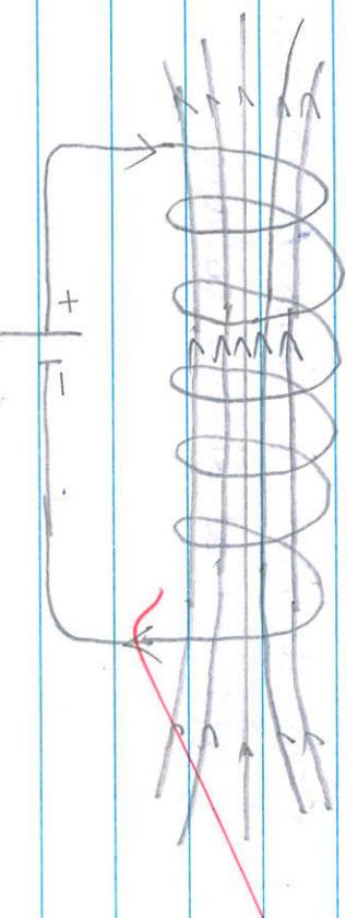
The magnetic field lines are straight and parallel to each other indicating that there is a uniform magnetic field inside solenoid.
