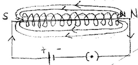
Magnetic field lines are maximum inside the solenoid and North-South around it.
