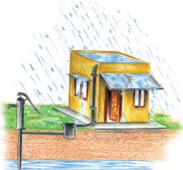
(a) Recharge through Hand Pump
